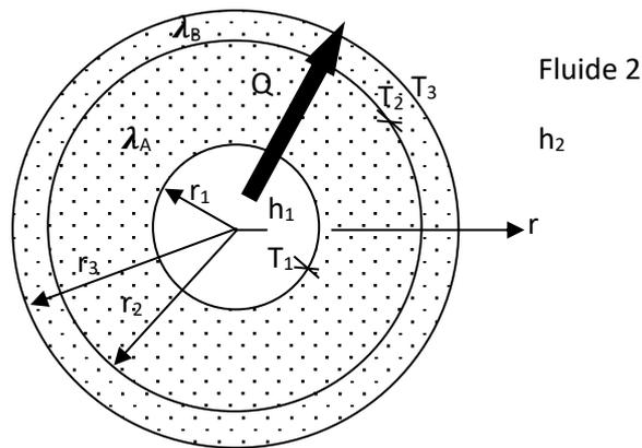
$$Q = 4\pi r_1^2 h_1 (T_{f1} - T_1) = \frac{4\pi\lambda_A (T_1 - T_2)}{\frac{1}{r_1} - \frac{1}{r_2}} = \frac{4\pi\lambda_B (T_2 - T_3)}{\frac{1}{r_2} - \frac{1}{r_3}} = 4\pi r_3^2 h_2 (T_3 - T_{f2})$$
