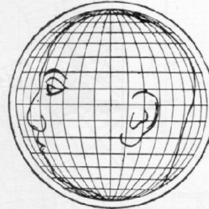
FIG. 44.—Man's head plotted on orthographic projection.
