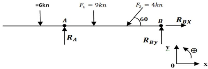
$$\sum_i \vec{F}_{\text{ext}} = 0 \Rightarrow \vec{F}_1 + \vec{F}_2 + \vec{Q} + \vec{R}_A + \vec{R}_B = \vec{0} \dots \dots \dots (I)$$
