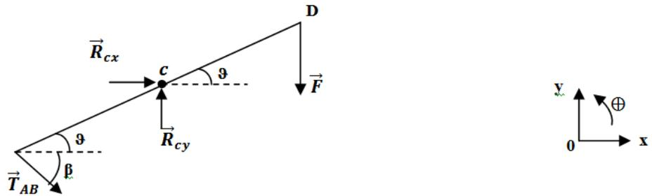
$$\sum_i \vec{F}_{\text{ext}} = 0 \Rightarrow \vec{T}_{AB} + \vec{R}_C + \vec{F} = \vec{0} \dots \dots \dots (I)$$
