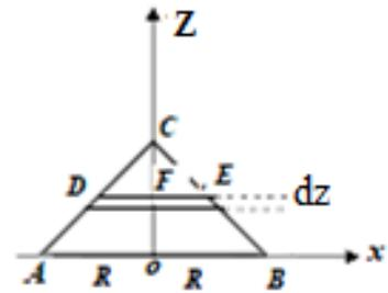
$$z_{2G} = \frac{1}{\sigma R^2} \int z \sigma dS_2 = \frac{1}{\sigma R^2} \int_0^R \sigma z \cdot 2(R-z) dz \Rightarrow z_{2G} = \frac{R}{3}$$
