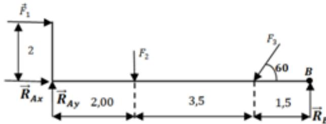
$$\sum_i \vec{F}_{\text{ext}} = 0 \Rightarrow \vec{F}_1 + \vec{F}_2 + \vec{F}_3 + \vec{R}_A + \vec{R}_B = \vec{0} \dots \dots \dots (I)$$
