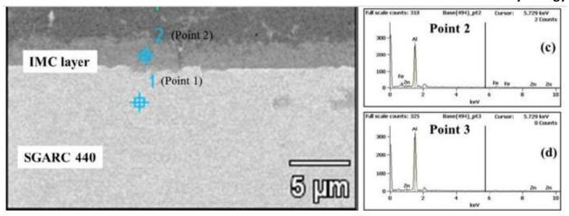
Energy dispersive X-ray spectroscopy (EDS) analysis locations in the welded section: (a) SEM image of dissimilar spot welds of aluminum alloy/zinc-coating steel.; (b) zinc-coating steel base metal point 1; (c) intermetallic compound (IMC) layer point 2; (d) aluminum alloy base metal point 3.
