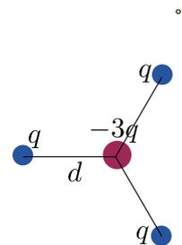
FIGURE 15.2 – Un quadripole pur.
