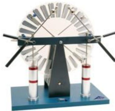
Figure 5: La machine de Wimshurst
