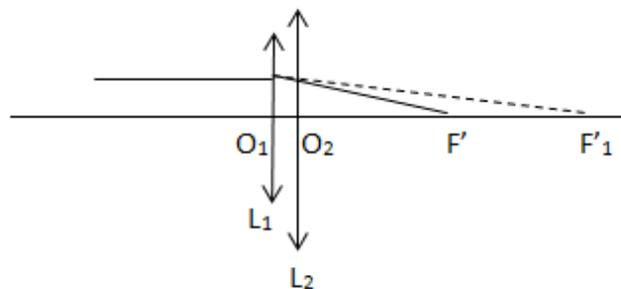
$$-\frac{1}{O_2F'_1} + \frac{1}{O_2F'} = \frac{1}{f_2} \text{ soit: } \frac{1}{O_2F'} = \frac{1}{f_2} + \frac{1}{O_2F'_1}.$$
