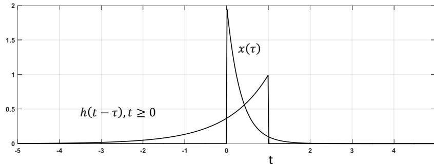
$$v_o(t) = \begin{cases} 0 & t < 0 \\ \frac{2}{3RC - 1} (e^{-t/RC} - e^{-3t}) & t \geq 0 \end{cases} \Rightarrow v_o(t) = \frac{2}{3RC - 1} (e^{-t/RC} - e^{-3t}) u(t)$$
