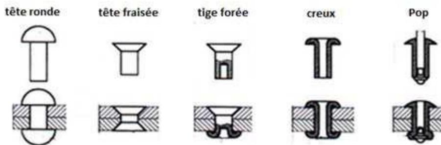
**Figure 5.4:** Types de rivets.
