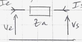
$$\left\{ \begin{array}{l} I_S = -I_e \\ V_S = V_e + Z_a \cdot I_S \end{array} \right.$$
